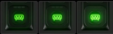
By firmware programming, both the color and the intensity of the light can be set for each LED. The same possibility also exists for the backlighting of the pushbutton.
