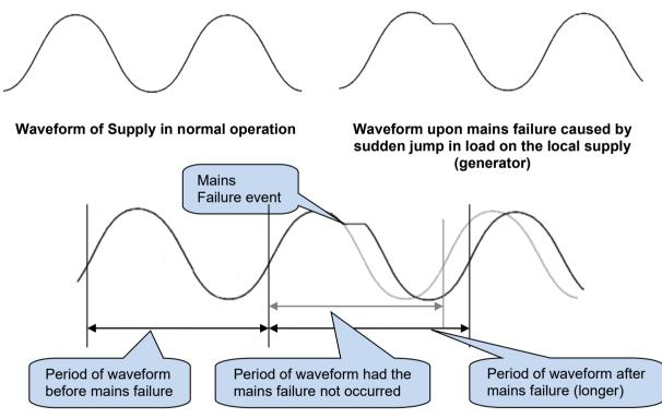
Waveform of connected supply overlaid with Waveform after mains failure
