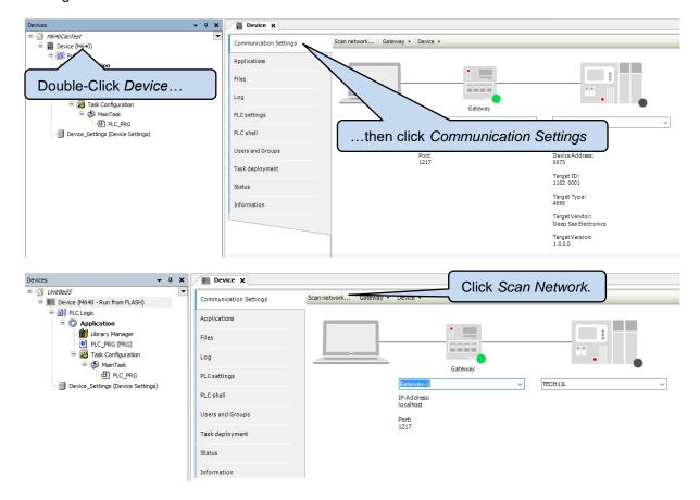
NOTE: A device in *Bootloader* mode is not discoverable by the Scan.
