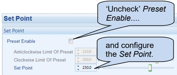
This allows the *Set Point* parameter to be configured.
