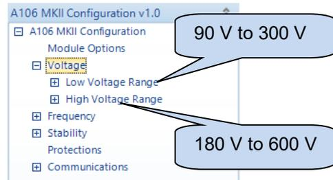
This voltage refers to the voltage applied to the AVR L and N (L2) terminals (the sensing voltage).
