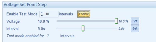
When the *Voltage Set Point Step* is activated the AVR first increases the excitation output voltage to increase generator output voltage. If this increase is too large, the set point is surpassed, requiring a decrease in excitation. The inverse of this process then occurs; the AVR decreases the excitation output voltage to decrease generator output voltage. As with the step-up, if the decrease is too large, the set point is surpassed, requiring an increase in excitation.
