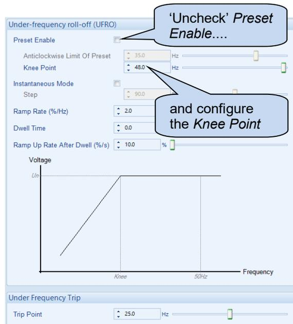
To ease setup, adjust *Knee Point* to a low value to prevent *Under Frequency Roll Off* from activating during the setup procedure.
