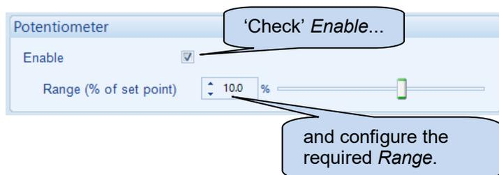
An open circuit (disconnected or damaged) potentiometer is automatically detected by the AVR and the output returns to the set point.
