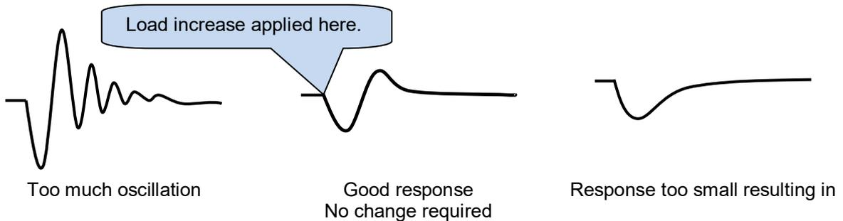
With the *Proportional* and *Integral* presets set as described in the procedure above, the initial response to the *Voltage Set Point Step* changes is likely to have been unstable. The next step to improve this response is to increase the *Derivative* preset.
