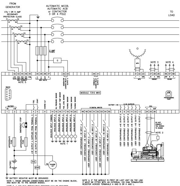
NOTE 2. A 120 OHM TERMINATING RESISTOR MAY BE REQUIRED EXTERNALLY, SEE ENGINE MANUFACTURERS LITERATURE.
