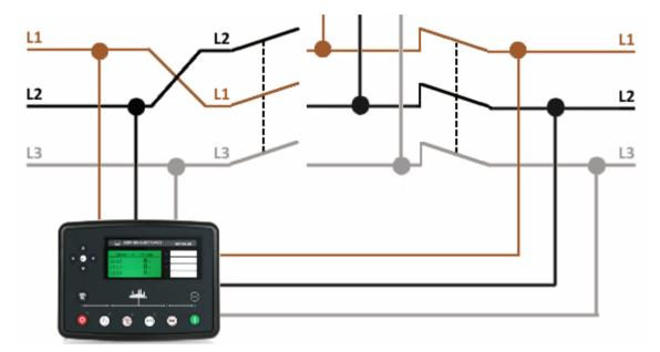
This is tested by starting the generator with the DSE module and ensuring the generator switchgear is left open (activate an input configured for *Generator Load Inhibit*). Then the load bus is to be made live, this is achieved by ensuring the mains switchgear is closed. Across the switchgear, connect a voltage meter to measure the AC voltage when the DSE module shows the two supplies in sync.
